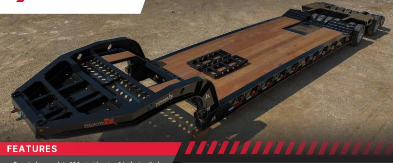
• Rear deck expands to 10 feet wide using 6-inch air cylinders
