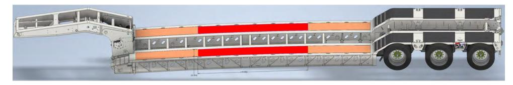
Notice: The load needs to be evenly distributed along the trailer deck, and evenly distributed across the support width of the trailer deck. Any point loading can cause premature damage to decking and buckling of crossmembers.
