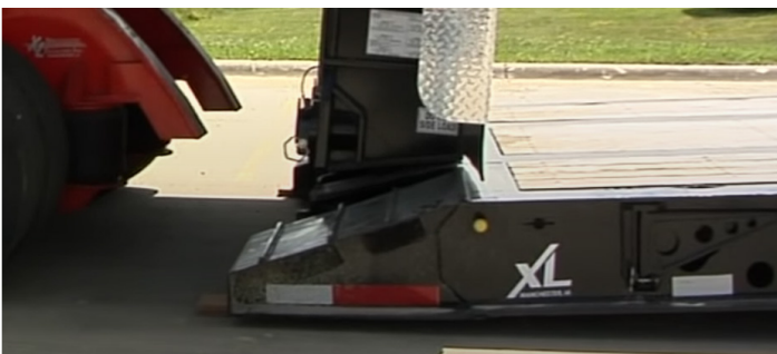
UNLATCH YELLOW HANDLE ON MAIN DECK
