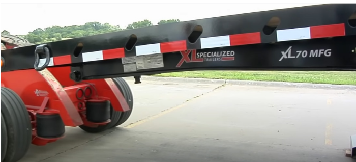
REMOVE 4X4 AND DRIVE CLEAR OF NECK
