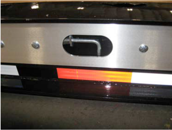
LOCK PIN IN LOCKED POSITION
