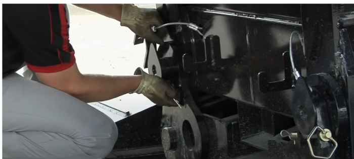
REATACH CONNECTOR PLATES & AIR/ELEC
