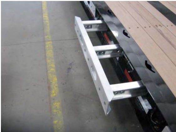
OUTRIGGER LOCKED IN TRAVEL POSITION
